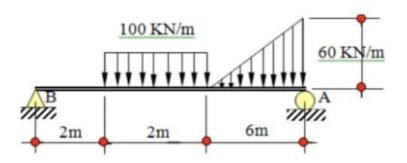
3. Determine the hinge reactions at point B and the roller reaction at A of the beam shown.
